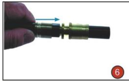
Insert fitting into expanded pipe to pipe stop, slide sleeve towards fitting.
