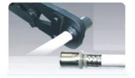
Open the handles and remove the pressing tool from the fitting and installation is accomplished.
