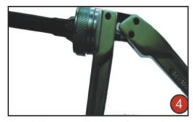
Insert the expander into pipe, make sure head Is square to pipe.
