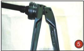
Expanding the pipe. Close levers of expanding tool, then release and rotate pipe slightly and repeat. This will ensure perfect roundness which will create a leak proof joint.
