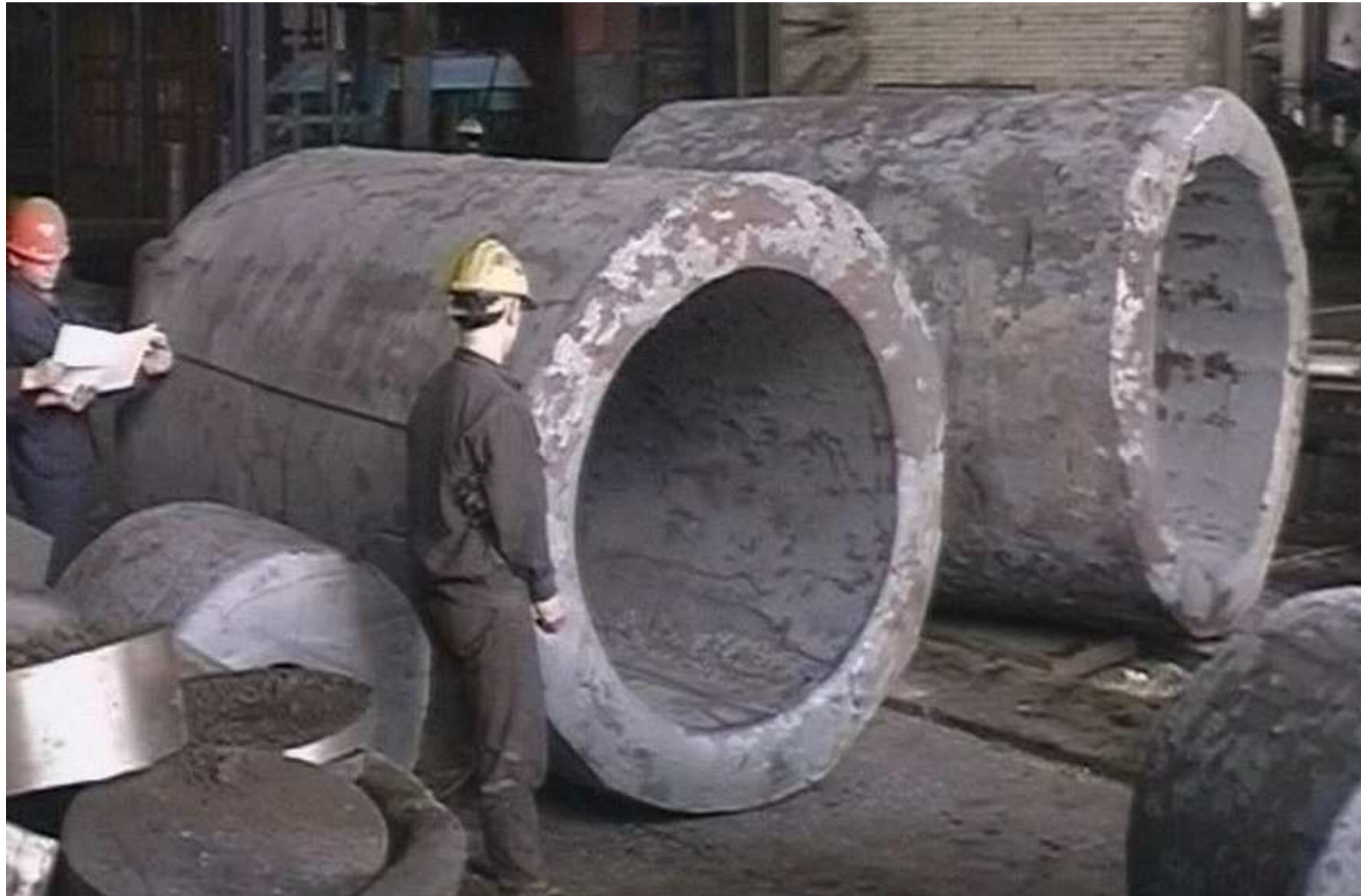
Forged barrel:outside diameter1800mm (Beiman)
