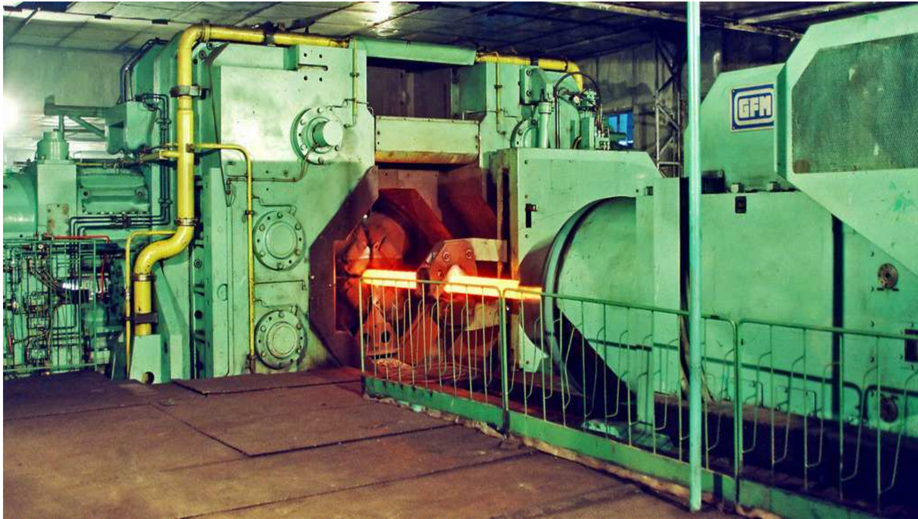
Fine forging press :1000t/GFM (Fushun)
