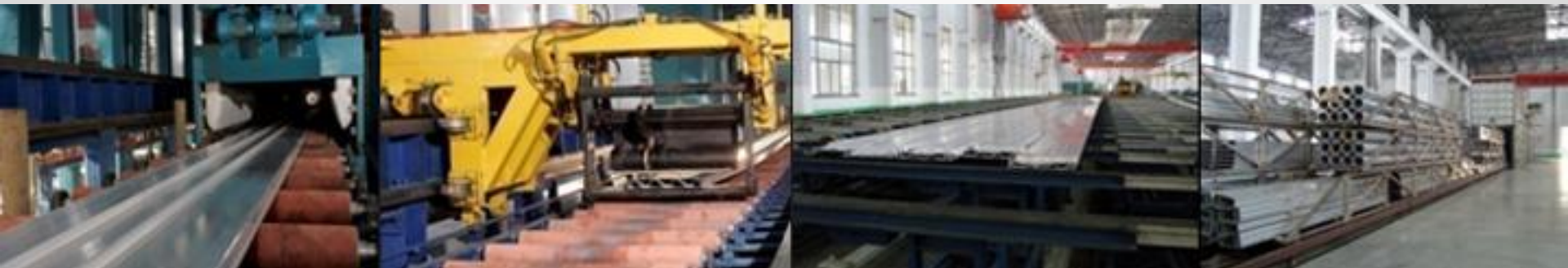
Stretcher leveling under 50^\circ\text{C} Stretch rate \leq 1.5\%
